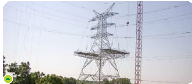
KPIL Twin Tower Testing facility in Gandhinagar, capable of testing up to 1,200 kV
