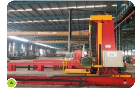
End Facing machine - Girder
