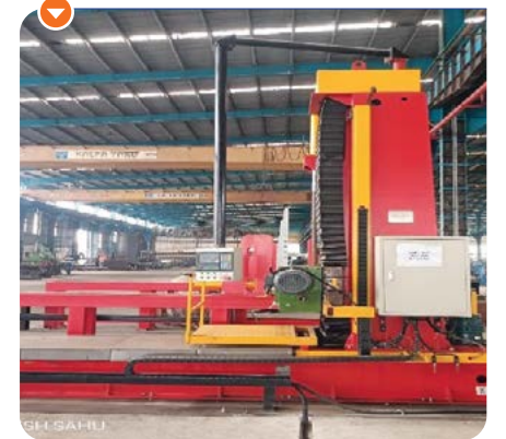
End-facing machine - Girder
